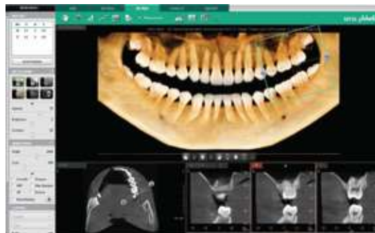
By clicking 3D Navigator and positioning to ROI, it's easy to verify 2D sectional images
